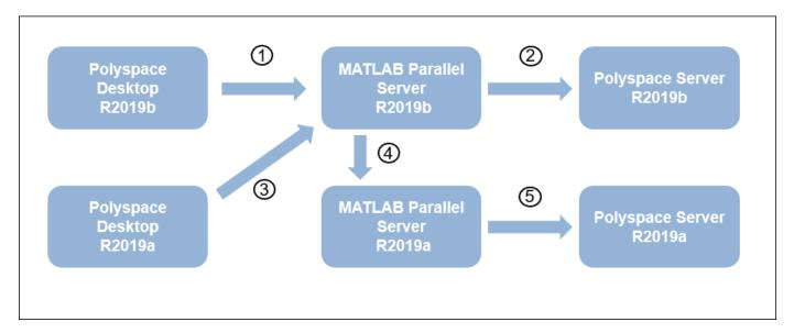
To support submissions from multiple releases with a single MATLAB Parallel Server cluster, you have to link the various installations of Polyspace products and MATLAB Parallel Server. Of the links shown in the preceding figure, the links numbered 1, 2 and 5 are part of a regular server-client installation using all products from the same release. To create all the links, do these steps:
